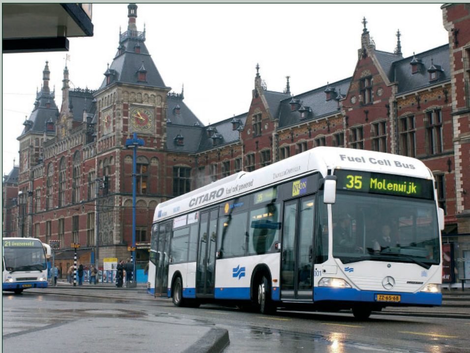
A bus in Amsterdam, powered by hydrogen, a fuel cell, and an electric motor.
