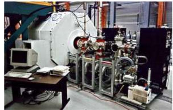
7T external electrospray FT-ICR setup at FOM-AMOLF. Indicated are three quadrupole ion guides, an open ended capacitively coupled ICR cell, the location of an electron gun for ECD several current probes to determine the ion optical transmission efficiency and the differential pumping stages with corresponding operating pressures. To bridge the gate valve between Q2 and Q3 an electrostatic Einzel lens is used consisting of GV1, GV2 and the gate valve housing as the electrodes.
