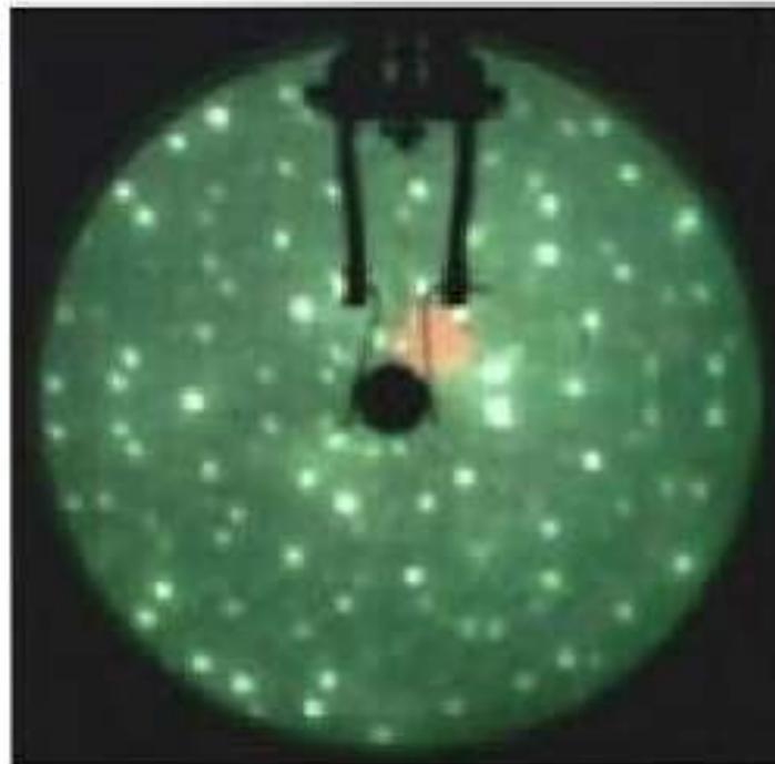
LEED images for sulfur adsorbed on Pd(111). A:  $(\sqrt{3} \times \sqrt{3})R30$  structure observed before heating and reconstruction, B :  $(\sqrt{7} \times \sqrt{7})R19.1$  surface reconstruction observed after heating.
